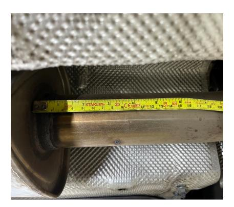
Measure 70mm back from the O.E resonator and cut the original exhaust at this point. The Scorpion pipe will fit over the original exhaust so ensure you remove all burrs from where you've cut the pipe.
